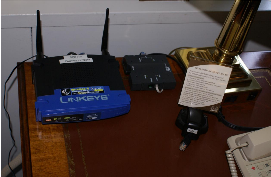
A device with two or more antennas is always a sign of a MIMO enhanced device.
