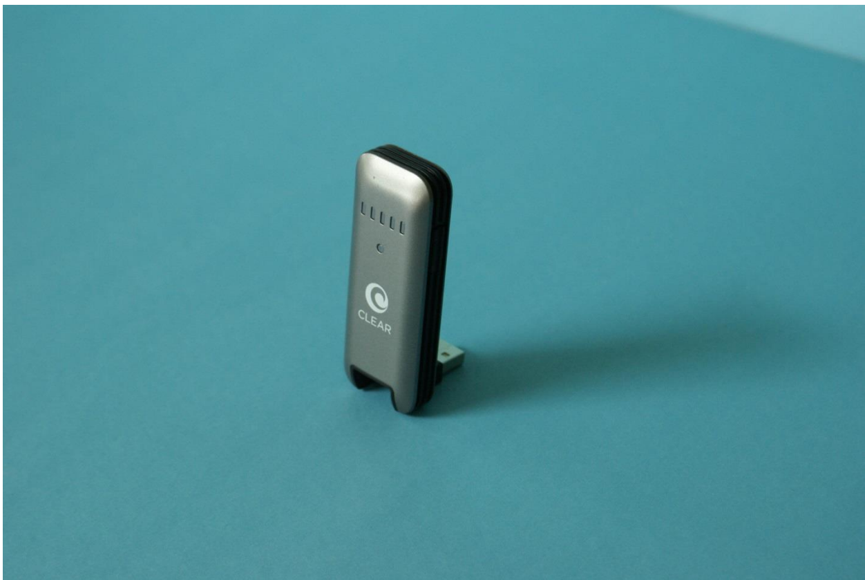
Mobile wireless broadband service can be added to a device through a USB port
